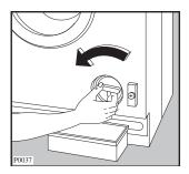
Unscrew and remove the filter.
